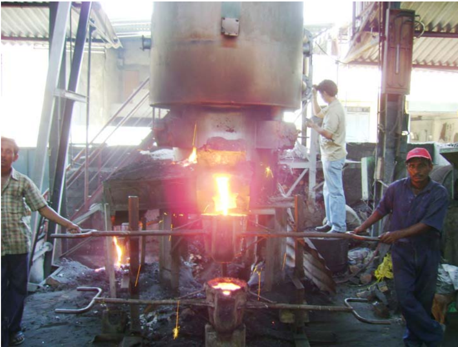
Foundry operation in Kolhapur cluster - Energy audit study revealed majority of installed Cupola are suboptimal kind, leading to higher fuel consumption
