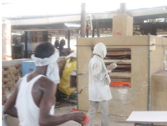
The Sikai Bhatti or Muffle Furnace in glass bangle making operation initially used to be coal fired and highly polluting. Figure shows a modified furnace after switching over to cleaner fuel
